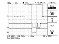
The routing unit passes control data bursts on to its slave devices.
